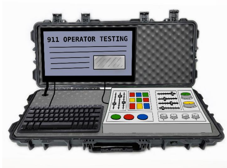
Figure 55: Conceptual sketch of the portable Taskbox designed by XXXX. A miniature keyboard, LCD screen, and Taskbox was designed to fit inside of a foldable case, thereby assisting in portability.
